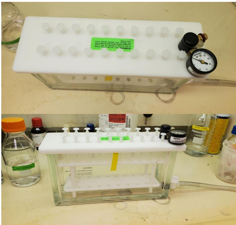
Figure 4: Displayed in the figure above is the top and side views of the vacuum manifold.
