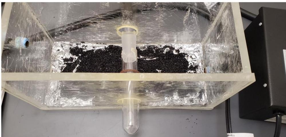
Figure 3: Displayed in the figure above is the PFOA loaded GAC distributed over the aluminum foil used to cover the bottom of the acrylic box and the UV-lamp and its protective sleeve fed through the holes.
