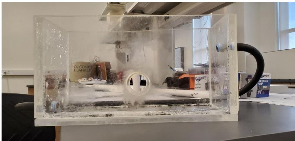
Figure 2: Displayed in the figure above is the acrylic box after the holes have been drilled in both of the long sides.
