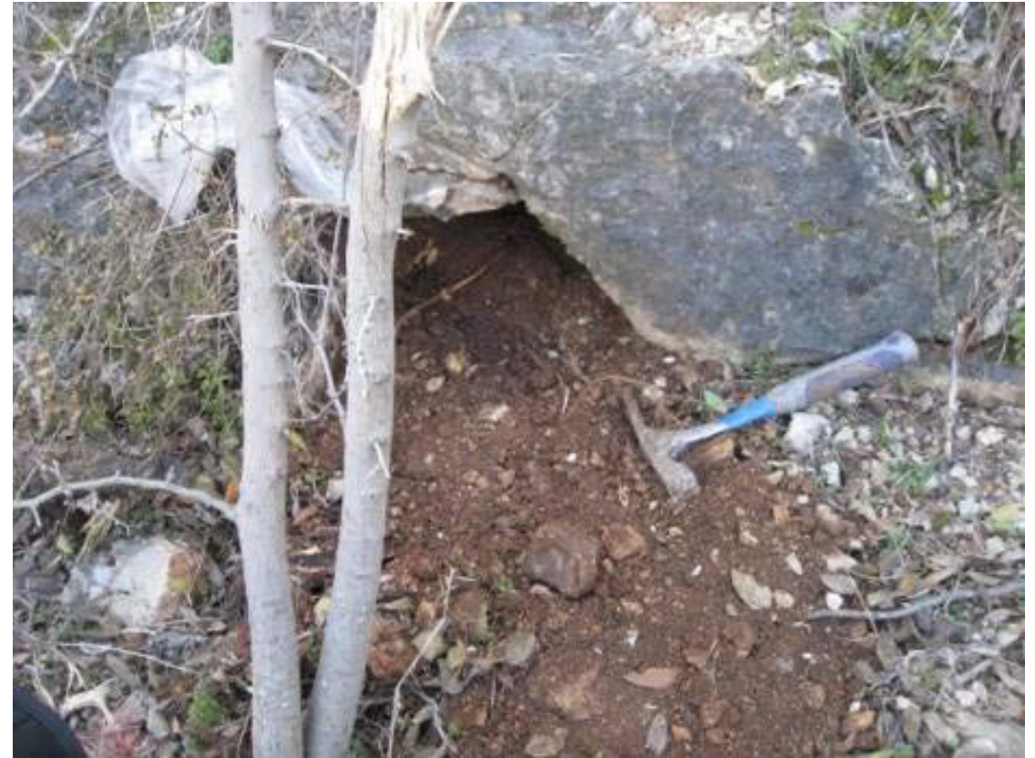
This cavity measures 1.5 x 1.5 ft and is 0.3 ft high The feature contains breakdown rocks, soil, and reddish brown clay.
